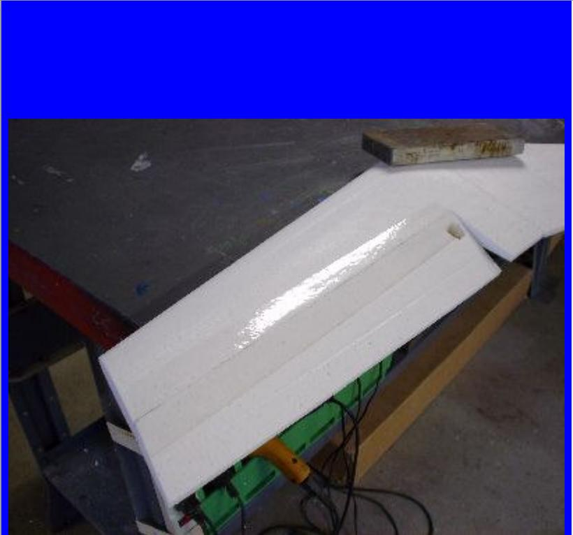
**6.** Then I stand the wing up (I use steel blocks to help hold it) and apply tape to the bottom of the hinge line, again half on the aileron and half on the wing. Burnish the tape down and trim the edges.
