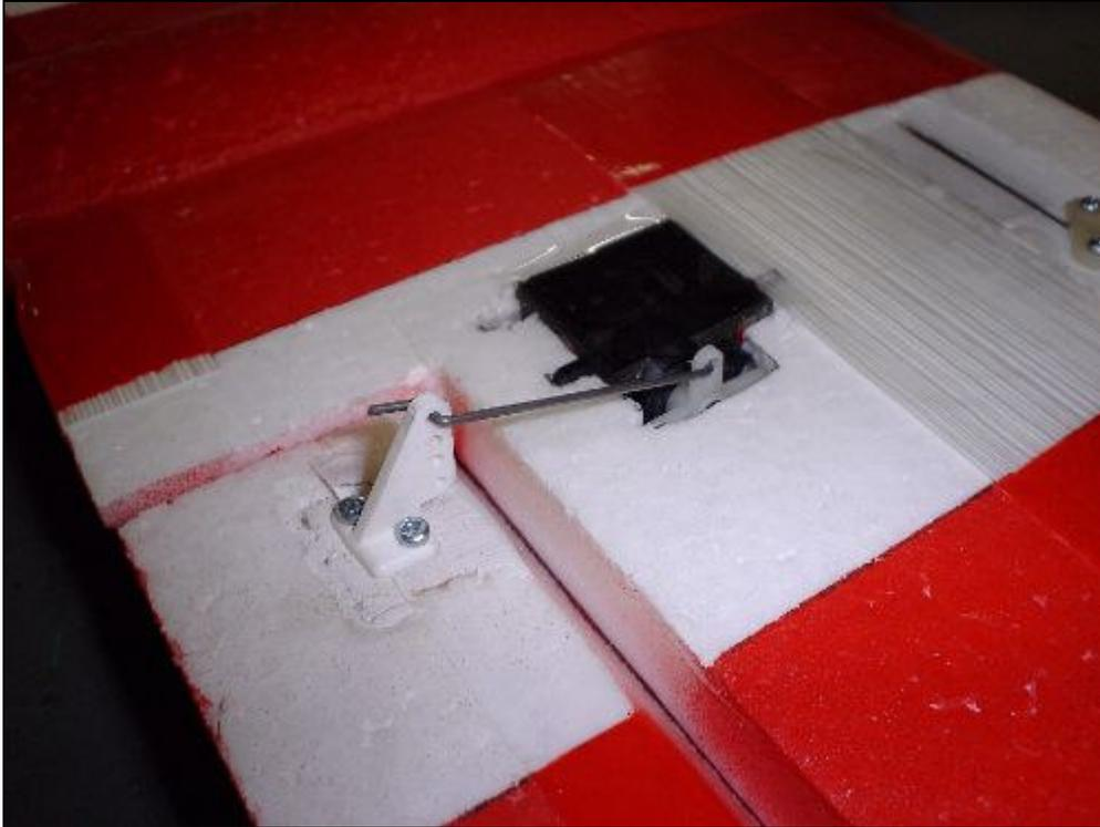
Here's the single aileron on my "Miss Swiss" plane. Notice this is the bottom of the wing. The servo (in this case a Hitec HS-81) is what I call "flat mounted" into a cavity in the foam with clear packing tape to secure it. Then there's the regular pushrod and control horn.
